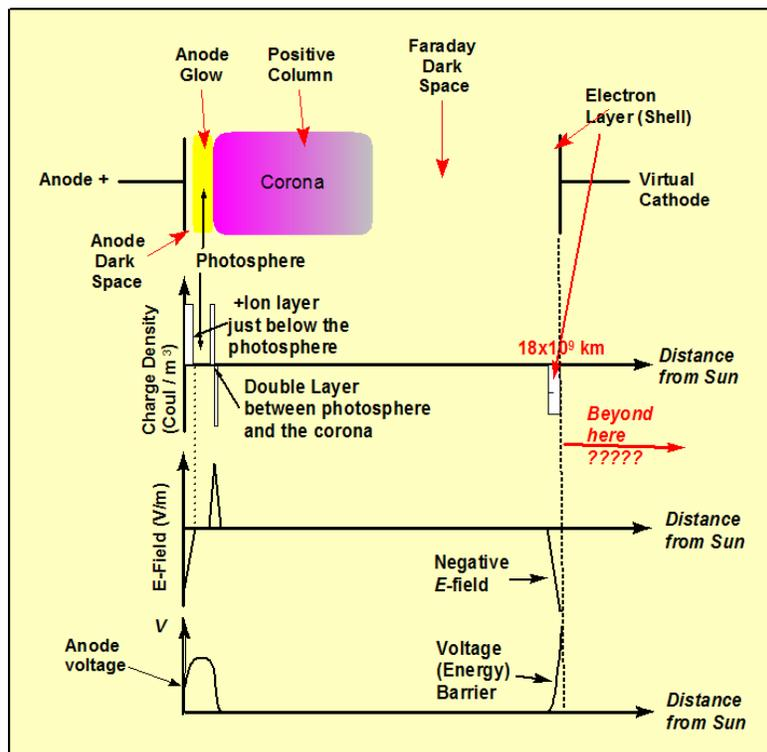
then the two lower plots show (by the same mathematical procedure as was used to derive the corresponding plots in figure 1) an increasingly strong negative electric field, and a voltage barrier for +ions.
