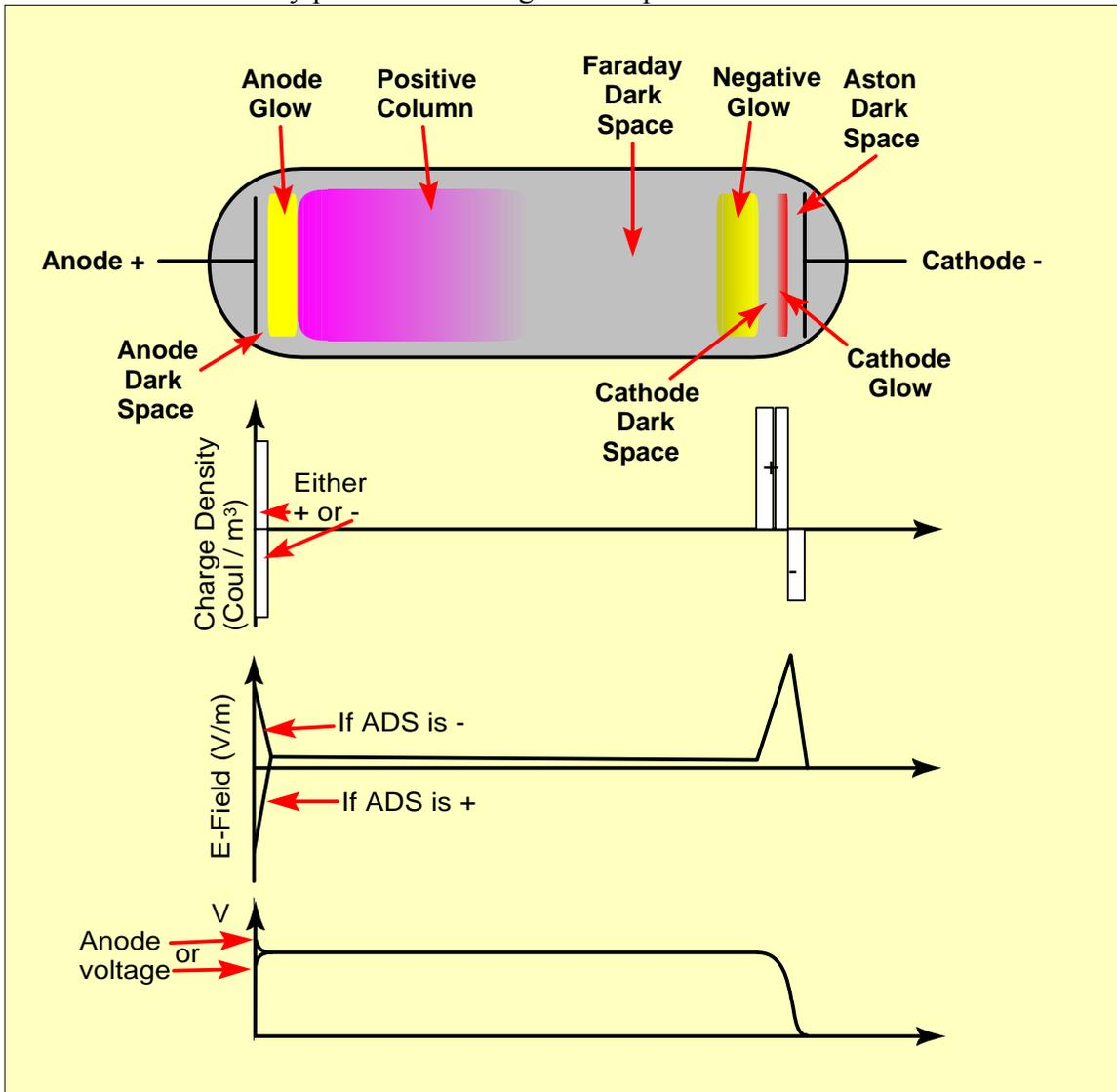
Figure 1. Classic structure of a plasma discharge in a laboratory setting.
