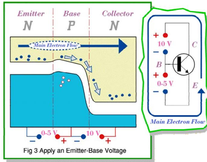
**Figure 3 Forward biasing the emitter-base junction reduces the height of the e-b barrier.**
