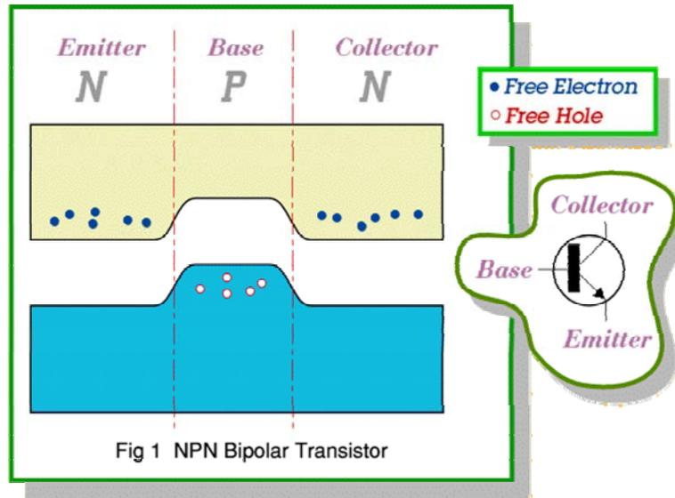
Figure 1. An unbiased npn transistor. The vertical axis is electric potential energy per unit charge (Volts).
