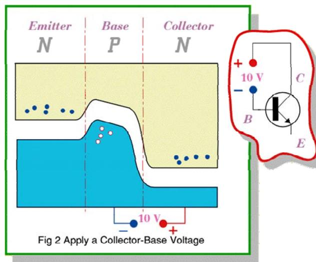
Figure 2 Back biasing the collector-base junction increases the height of the c-b barrier. (Credit: The Scots Guide to Electronics<sup>iii</sup>)
