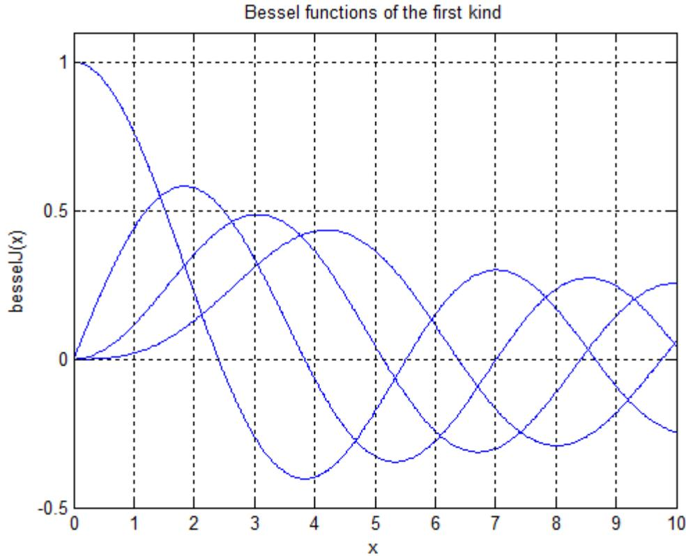
Figure 3. Bessel Functions<sup>vii</sup> of the first kind,  $J_0$  through  $J_3$  are closed-form solutions of equations 9 and 17.
